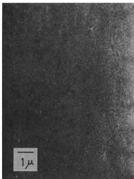
Fig. 3. Scanning electron micrograph of the surface of the microporous film, no. 1.
